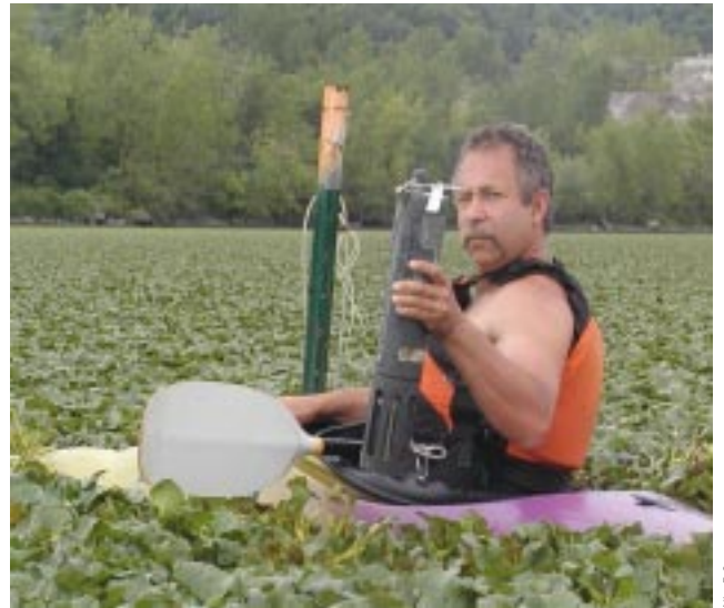
Dr. Jonathan Cole retrieving a sonde meter from a water chestnut bed in Inbocht Bay, NY. Sonde meters are used to record dissolved oxygen, pH, turbidity, temperature and depth in aquatic systems.
