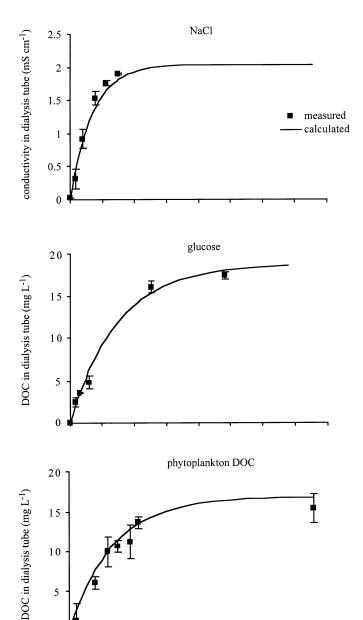
Fig. 1. Measured and calculated conductivity or DOC concentration in the dialysis tubes over time from exchange experiments with NaCl, glucose and phytoplankton derived C. Error bars show  $\pm 1$  SD.
