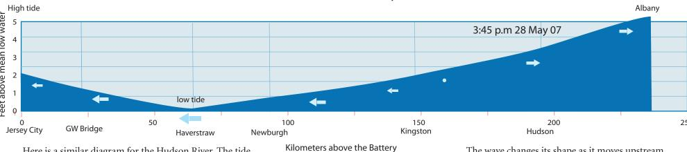
Here is a similar diagram for the Hudson River. The tide Kil moves 235 kilometers in 8.75 hrs, or about 26 kilometers per hour or 16 miles per hour. The wave changes its shape as it moves upstream, somewhat like a wave moving up a beach. In the upper river tides rise fast and fall slowly.
