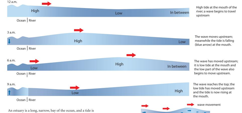
An estuary is a long, narrow, bay of the ocean, and a tide is a long wave moving up it. The speed of the tidal wave, in miles per hour, is roughly 4 times the square root of the depth in feet. If, for example, the high tide moves 100 miles upstream in 6 hours, for a speed of about 16 miles an hour, the average depth must then be  $(16/4)^2$ , or 16 feet.
