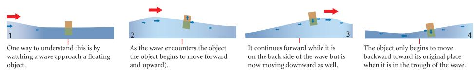
Thus the direction an object (and hence the current it is in) moves doesn't tell us whether it is on the rising or the falling part of the wave. In panels 2 and 3 the object is moving to the right, but in panel 2 the object is on the rising part of the wave, and on panel 3 the falling part.
