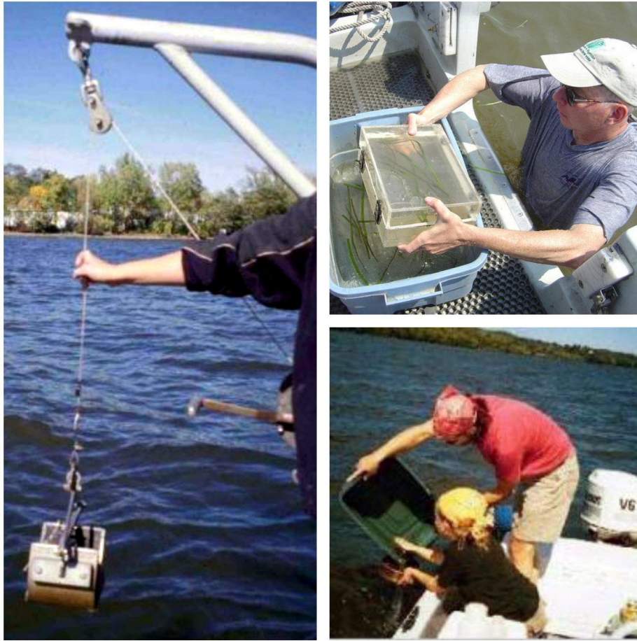
Clockwise from left: A PONAR grab ready to deploy; Dr. Dave Strayer bringing a Downing Box sample up onto the boat; Researchers using a sieve to remove macroinvertebrates from sediment samples.
