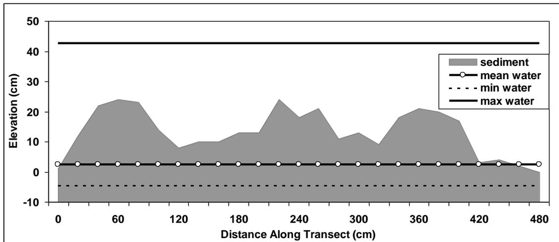
**FIGURE 2.** The topographical profile for site one transect 25 m from the channel is shown in gray. Maximum, mean, and minimum water levels observed from June 29 to July 8, 2009 are indicated by the horizontal lines. All water levels are relative to the lowest point on the transect which has a value of zero.
