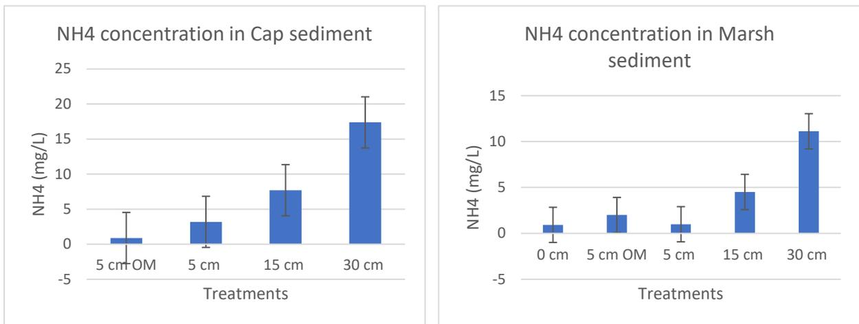
**FIGURE 4.** The graph to the right corresponds to the NH<sub>4</sub> concentration in porewater of marsh sediment. The graph to the left corresponds to the NH<sub>4</sub> concentration in cap sediment.
