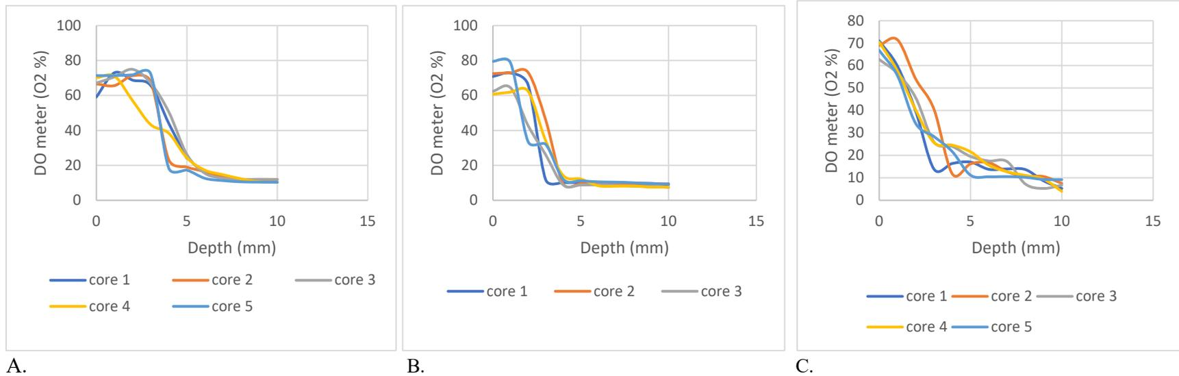
**FIGURE 2.** A. Oxygen profile for control treatment, no cap sediment added. B. Oxygen profile for treatment with 5 cm cap added. C. Oxygen profile for treatment with 5 cm cap added and extra organic matter (OM).
